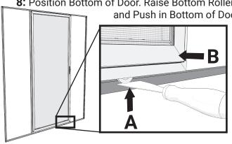
9: Adjust Rollers For Smooth Operation. Bottom Rollers Before Top Rollers
