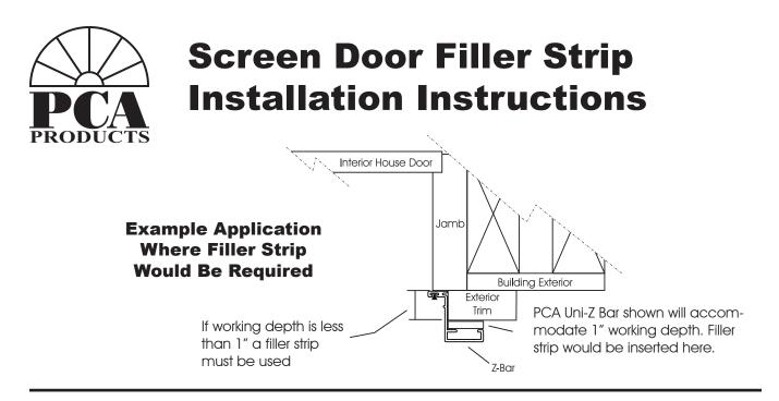
Installer must "prep" the z-bar with filler *BEFORE* installing in opening. Filler will need to be attached to all three pieces of z-bar. (2) Left and right z-bar legs and (1) Z-bar header
