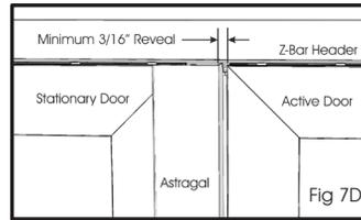
**E:** Secure Astragal with a total (4) #8x1/2" tek screws from the inside. **IMPORTANT: Stay at least 4 inches from top and bottom of door frame to avoid hitting the internal corner key!** (Fig 7E).
